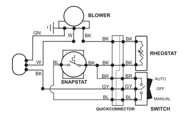
Figure 37. Blower Wiring Diagram
